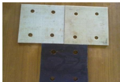
Fig 1 Glass fiber epoxy, Glass fiber polyester and Mild steel
