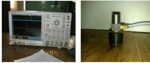
Fig 2 Digital Storage Oscilloscope of Tektronix 4000 series and Vibration pickup
