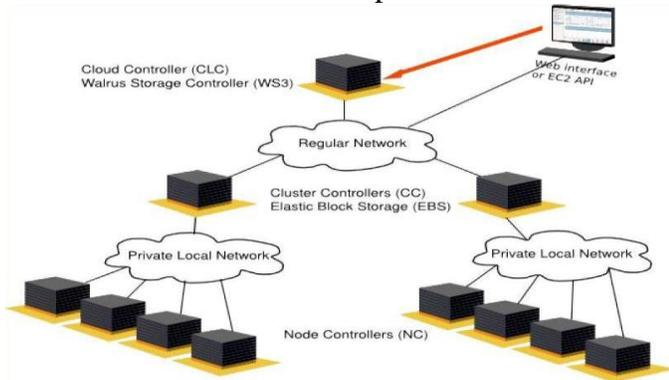
**Figure 3.1: Architecture of Ubuntu Enterprise Cloud**
