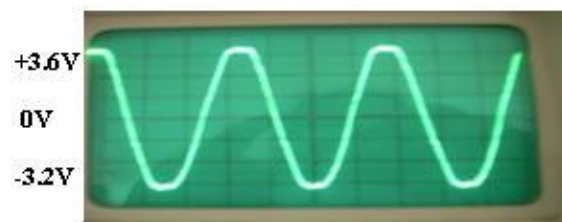
Fig.17 Voltage waveform after switching ON of Lamp load
