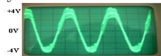
Fig.18 The compensation Voltage waveform after switching ON of the DVR when the DVR is ON. The obtained sag is compensated the compensation of voltage waveform with clear graphical fluctuations are shown in the fig. 18.
