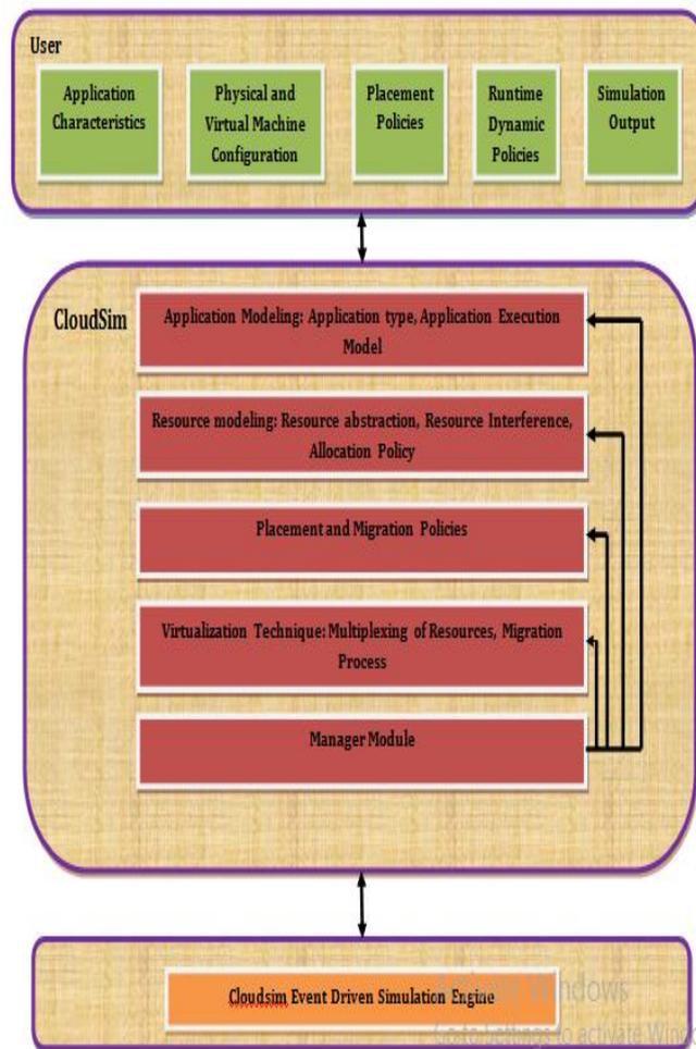
**Figure 2: Block diagram of CloudSim [2]**
