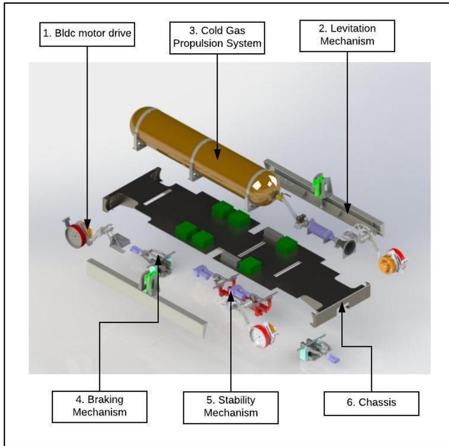
**Fig. 1. COEP Hyperloop system architecture.**
