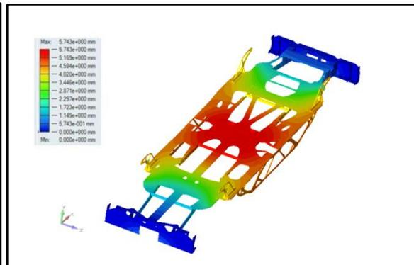
**Fig. 6. Displacement contour: optimized chassis**
