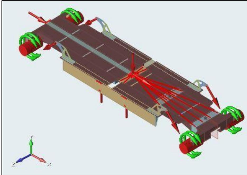
**Fig-3. Free body diagram of the chassis**
