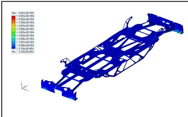
**Fig. 5. Von Mises stress contour: optimized chassis**
